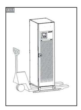
To facilitate handling, two yellow skis (700mm) are screwed onto the feet, in the widthwise direction The cabinets can be handled from underneath using a pallet truck or forklift truck, with the forks introduced from the sides only. Remove the side grids of the cabinet, then position the forks underneath it:
