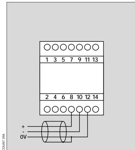
The Countis Ci can be connected to an RS485 communication network with JBUS/MODBUS® protocol. For a standard configuration, 31 Countis Ci may be connected over a distance of 1500 metres (9600 bauds). Should the distance or maximum number of
